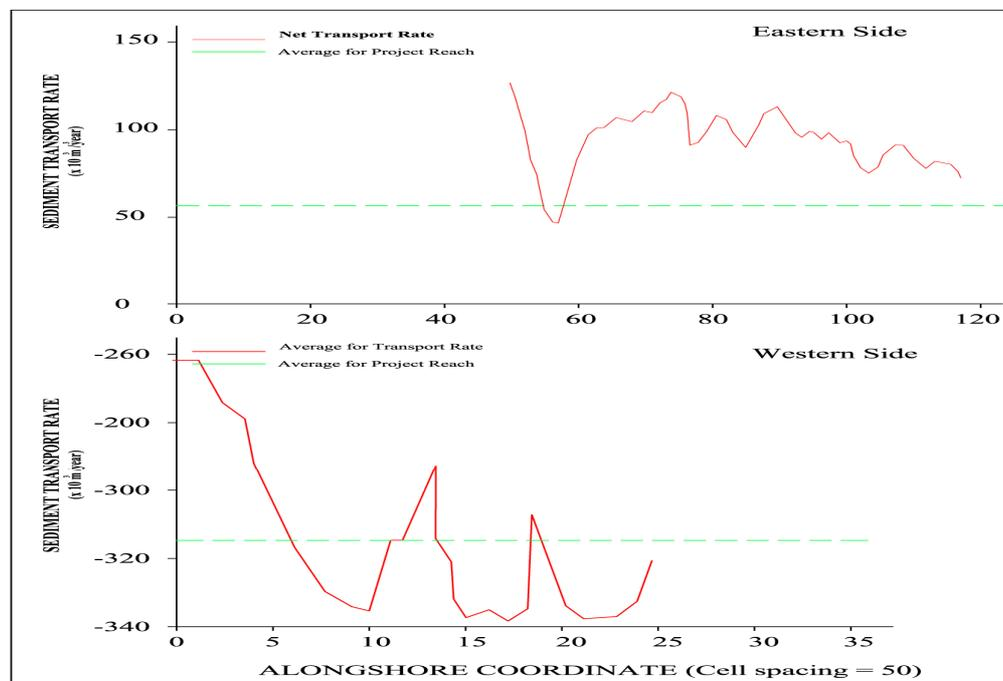
**Fig. 5.** Rate of sediment transport along Rosetta area 1996/1997 ( $\times 10^3 \text{ m}^3$ )
