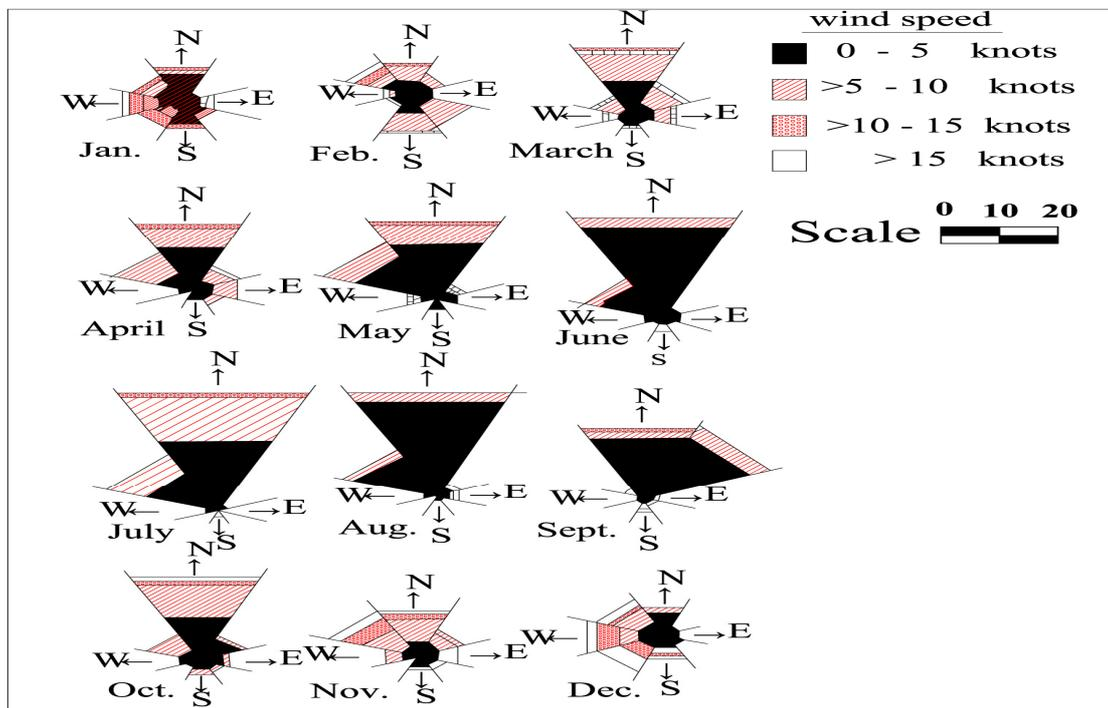
**Fig. 3.** Monthly wind rose diagram – Rosetta area
